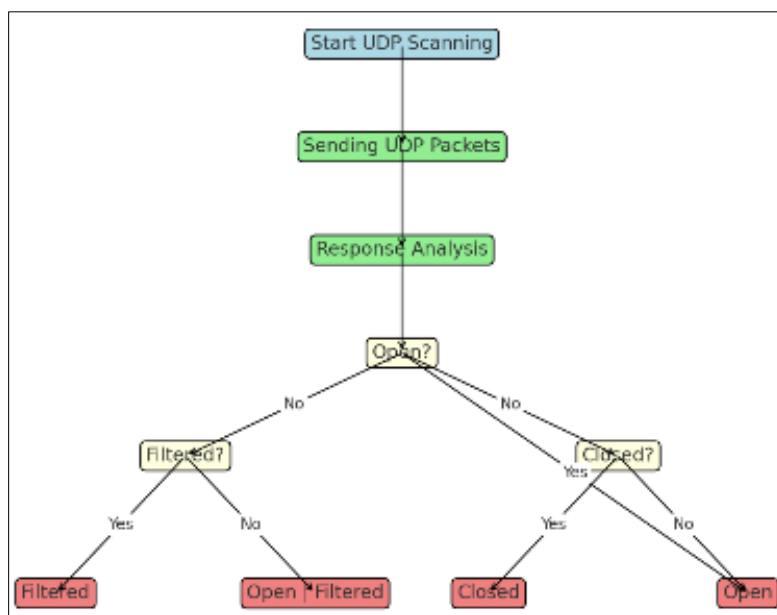
Figure 3 Flow chart of the UDP scanning process (Jung et al. , 2021)
