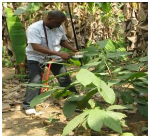
Figure 1 Infra-Red Gas Analyser (IRGA) being used in Ibadan to collect photosynthetic rate, stomatal conductance and stomatal transpiration at \geq 300 \mu\text{mol m}^{-2}\text{s}^{-1} of sunshine needed for optimum performance of cocoa
