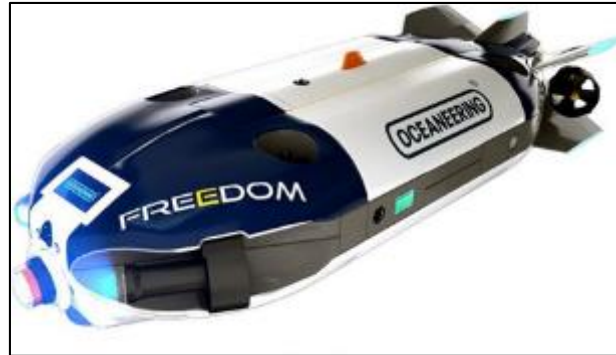
Figure 1 The Freedom ROV, a type of Remote Operated Vehicle used in complex, hazardous environments like unconventional reservoirs. [5]
