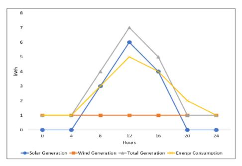
Figure 1 Average Hourly Energy Generation and Consumption (kWh)
