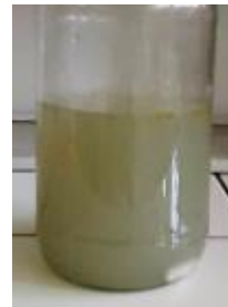
Figure 3 Sample of 259 NTU treated with the solution obtained of vegetable oil from soursop seeds
