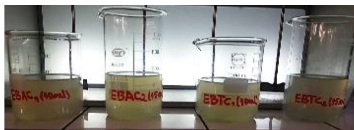
Figure 9 Sample of domestic wastewater of 160 NTU treated with the solutions obtained of almond and integument ashes from soursop seeds
